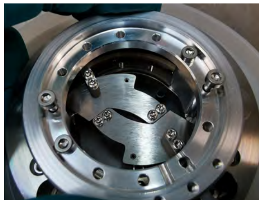
Fig. 2: Collimator with unilaterally cooled blades driven by one linear actuator, arrangement with a small aperture (2 of 4 blades visible) (Credit: Frieder Müller).
