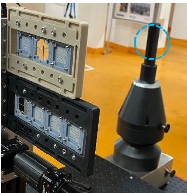
Fig. 1: Fluorescence detector (blue circle) at the ARES accelerator at DESY during FLASH therapy studies.
