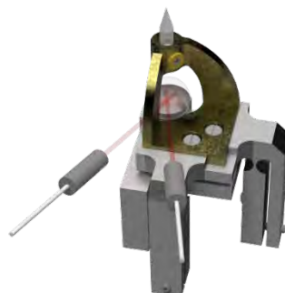
Fig. 2: Sample holder with laser.
