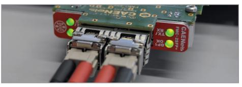
**Dual-channel FMC-SFP+ version during operation**
