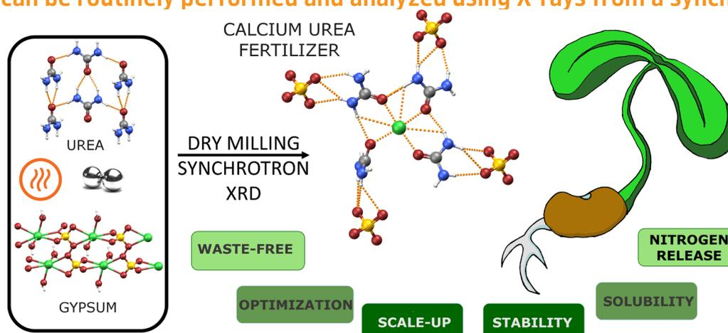
**FIGURE 1** | Milling gypsum and urea with steel balls creates a so-called co-crystal that releases its nitrogen only slowly. (Credit: Ruđer Bošković Institute, Krunoslav Užarević)
