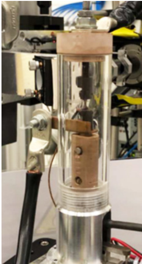
Figure 1: Custom load frame used for SAXS, 3DXRD and tomography of nickel superalloys. A Joule heating system is also included. Copied from Vinnova project report number 2019-02584.
