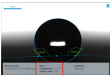
Imaging from the contact angle measurements: The drops remain spherical on the textile surface at a contact angle of 140° and hardly adhere to it (Images: research consortium)
