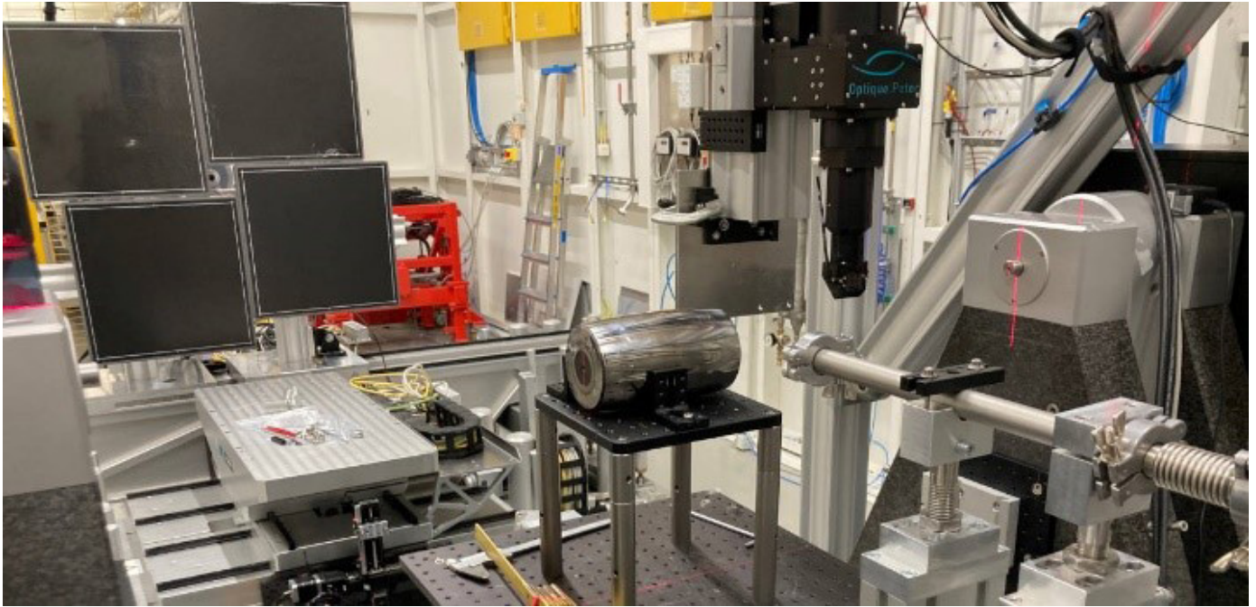
Figure 1: Left: Setup of the sample in the beamline. The beam enters through the stainless tube (lower right) cuts through the roller (middle) and is caught by four large area detectors (top left).
